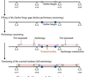
Figure-3 Steps to full tensioning
